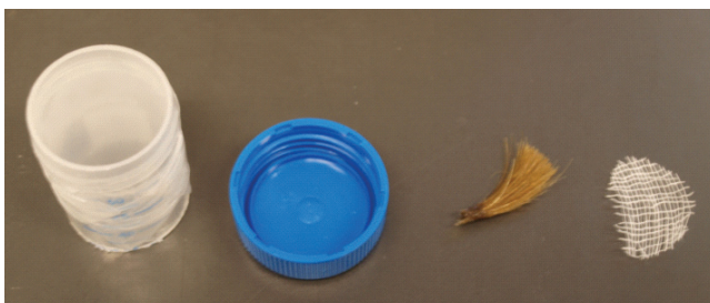
Figure 2. All components of the in vitro rearing unit; rearing vessel, blood reservoir, hair tuft and piece of wide mesh gauze.
